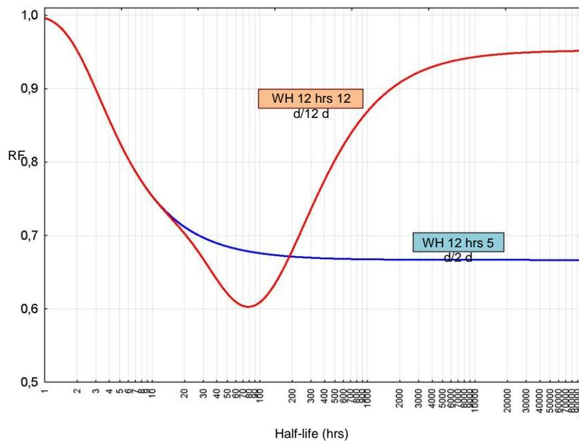
**Figure 9:** The dependence of the reduction factor (RF) on the half-life and the number of working and free shifts according to formula (5) from Hickey and Reist (1977). In both cases, however, the working time is 12 hours, in one case 5 working shifts and 2 days off, in the other case 12 working shifts and 12 days off
