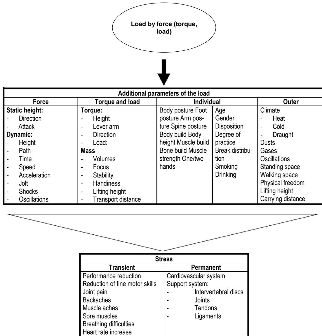
**Figure 6:** Load and stress factors due to the application of force (Hecker R., 1998)
